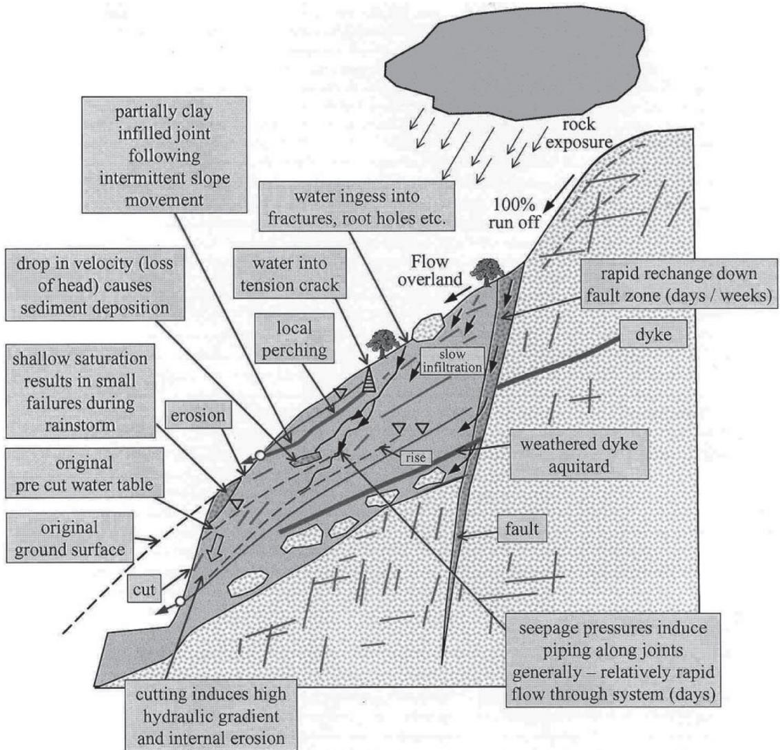
Figure 17. Hydrogeological mechanisms - each with its own time frame
