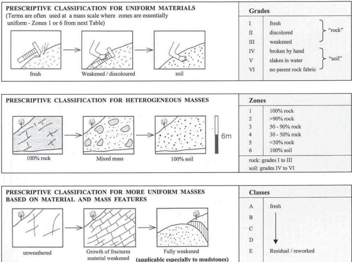
Figure 13. Prescriptive weathering classifications (simplified from Anon, 1995)
