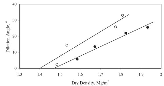
14b. Dilation angle vs dry density of sample for given normal stress levels
