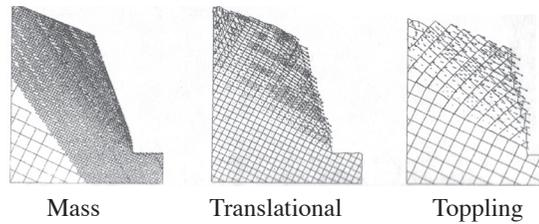
Figure 2. UDEC models showing changing style of failure, dependent solely on discontinuity spacing (after Hencher et al 1995)
